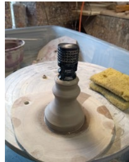
3D printed tap & die (~18mm).
