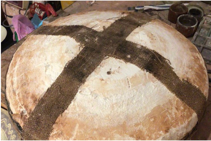
Fruit bowl mould with strengthening
