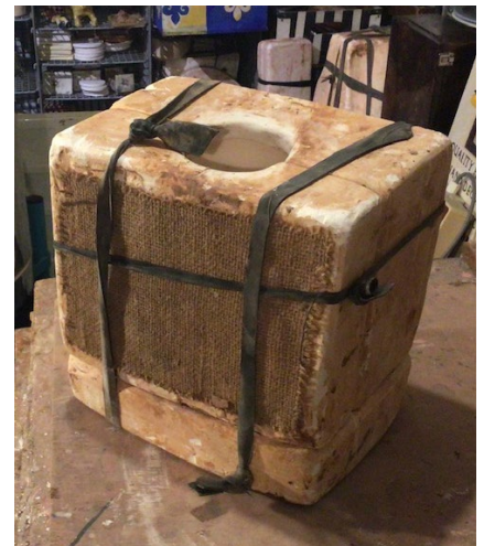
Strapped tankard mould
