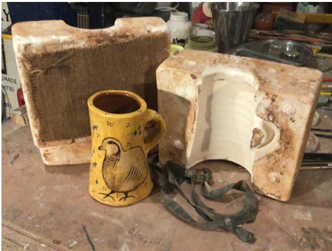
Mould with hessian and inner tubes with a finished slip cast tankard
