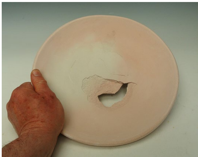
Plate casualty caused by bisque firing before the bone dry state was reached
