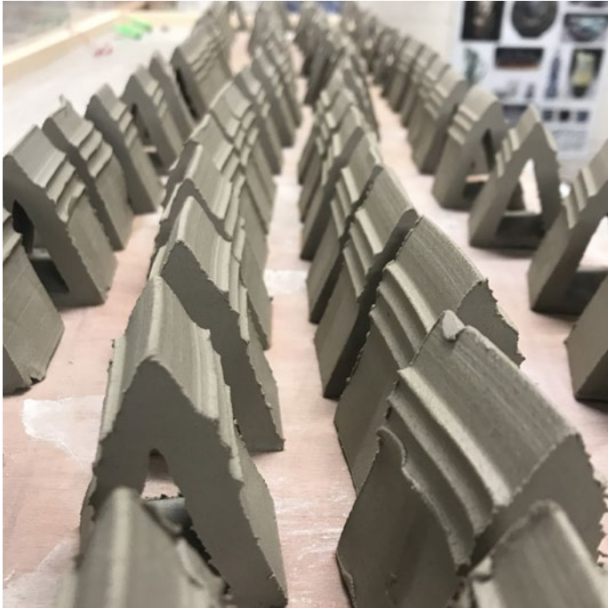
Extruded test tiles using grogged stoneware
