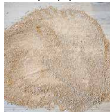
R2 in need of further crushing
