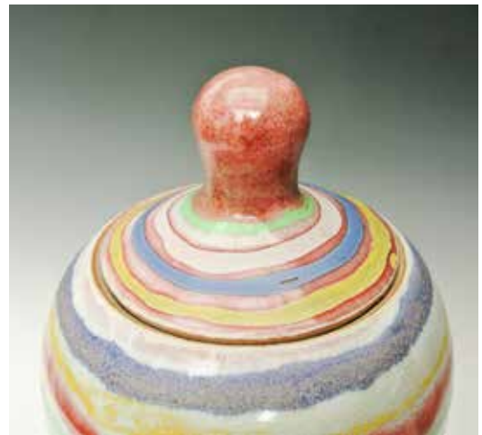
Detail of a jar showing softer pinks where copper is evaporating from one glaze and colouring another. Copper is very volatile at earthenware temperatures and more so at stoneware temperatures. This is why the copper red glaze needs thick application as the copper from a thin layer will disappear up the flue with the exhaust gases.
