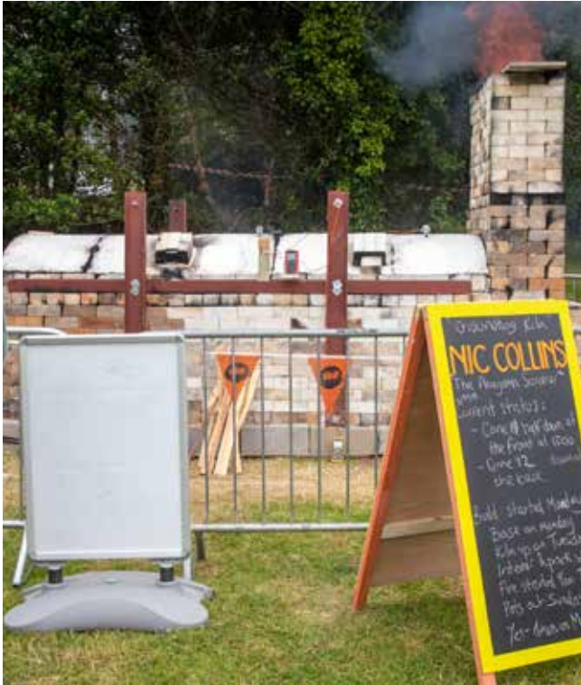
Nic Collins: Ground hog type wood fired cross draft kiln, constructed on site, packed, fired over 36 hours to cone 12 throughout, cooled down in 12 hours and then dismantled. All the pots survived.
