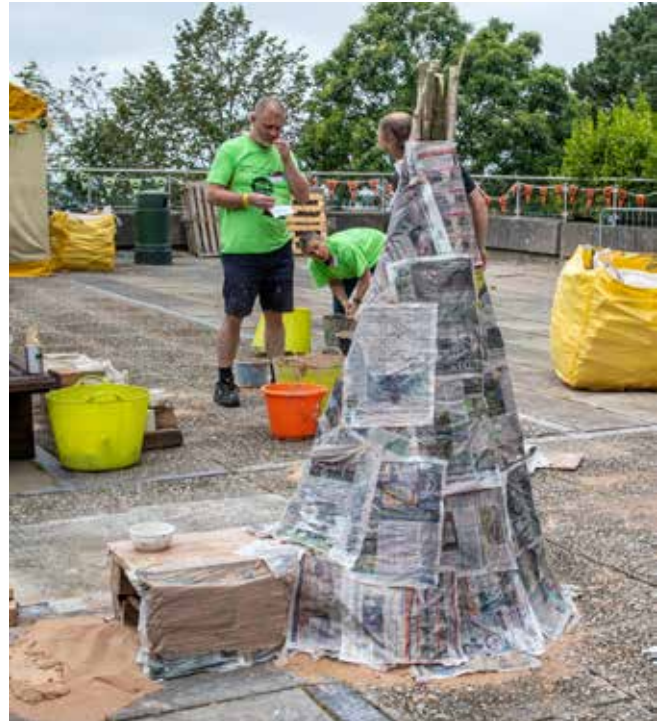
Terry Davies: Tipi kilns made of cotton, paper and clay round a frame of thin branches, to be fuelled by wood
