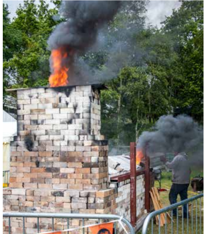
Nic Collins: Ground hog type wood fired cross draft kiln, constructed on site, packed, fired over 36 hours to cone 12 throughout, cooled down in 12 hours and then dismantled. All the pots survived.
